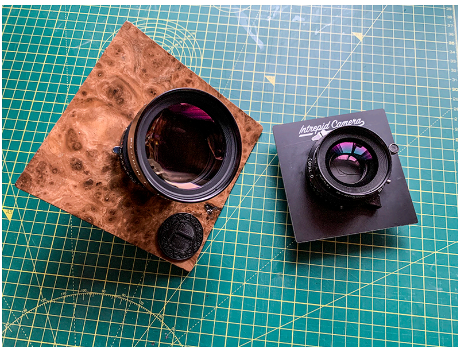
Note the 10x8 lens board and 300mm lens on the left and 5x4 lens board on the right with 150mm lens.
